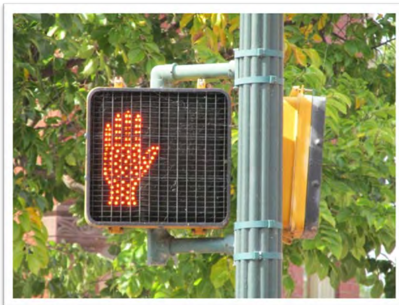
Pedestrian signal head in Harrisburg City
