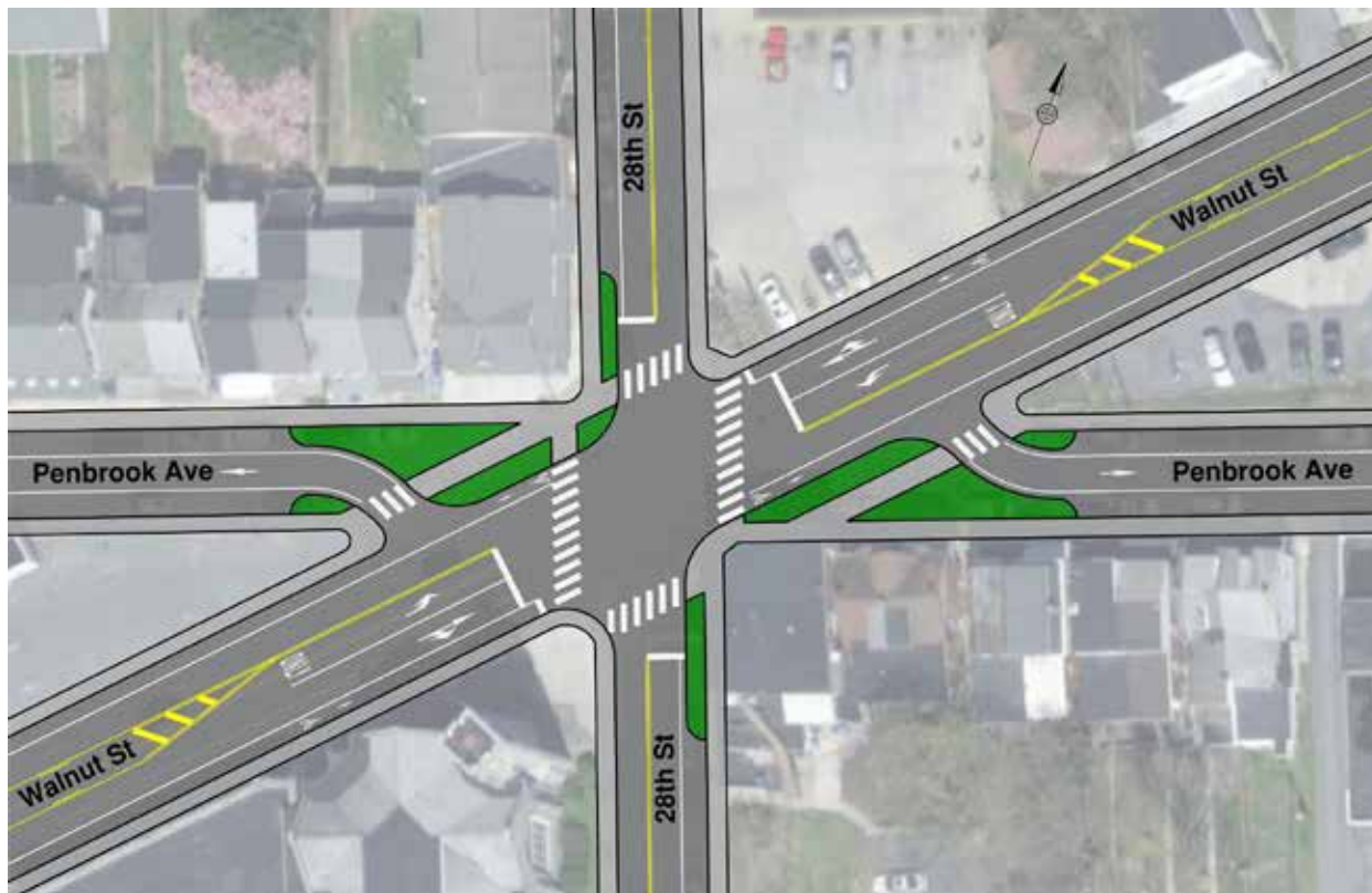
Road diet and geometric configuration for Walnut St and 28th St and Penbrook Ave intersection
