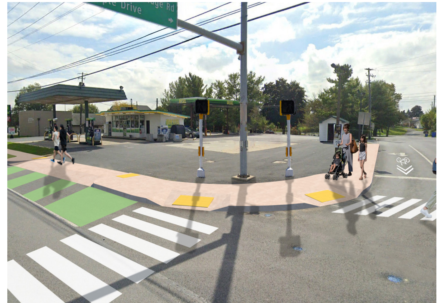
Rendering depicting proposed short and mid-term improvements for the Corridor. The addition of sidewalks, bikelanes, high-visibility crosswalks, and pedestrian signals can be seen. These improvements are proposed throughout the Corridor.
