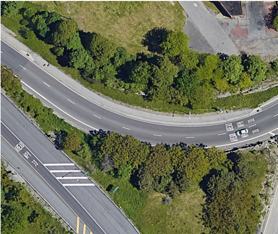
Figure 22 – Reduced Speed Ahead Pavement Markings, NY 198 at NY 33 Interchange, Buffalo, New York
