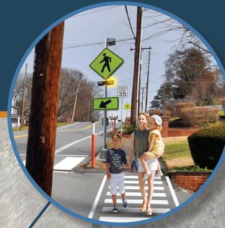
Crosswalks and rapid flashing beacons at School St. & Sunbury St.
